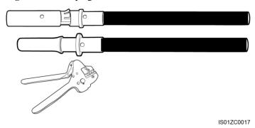
**Step 3** Insert the crimped positive and negative power cables into the corresponding positive and negative connectors until they snap into place.
