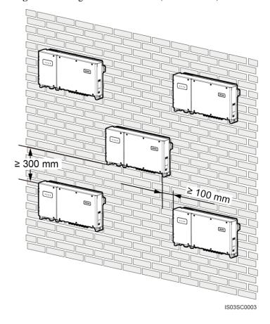
Figure 4-6 Triangle installation mode (recommended)
