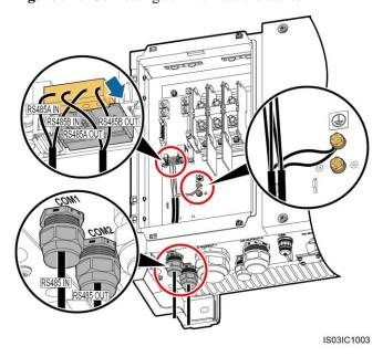
Figure 5-29 Connecting communications cables
