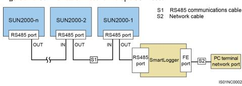
Figure 5-25 Communication mode for multiple SUN2000s
