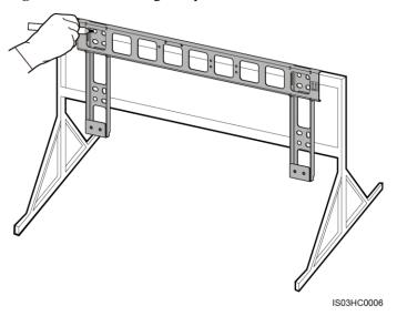
Figure 4-24 Determining hole positions
