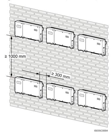
Figure 4-7 Stacked installation mode (not recommended)
