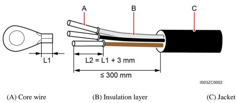
**Figure 5-9** Four-core cable (including the ground cable but excluding the neutral wire)
