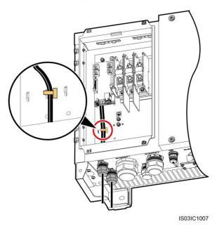
**Step 8** Use a torque wrench with an open end of 33 mm to tighten the locking caps to a torque of 7.5 N m.
