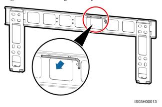
**Step 2** Determine the positions for drilling holes using the mounting bracket available in the packing case. Level the hole positions using a level, and mark the hole positions using a marker.
