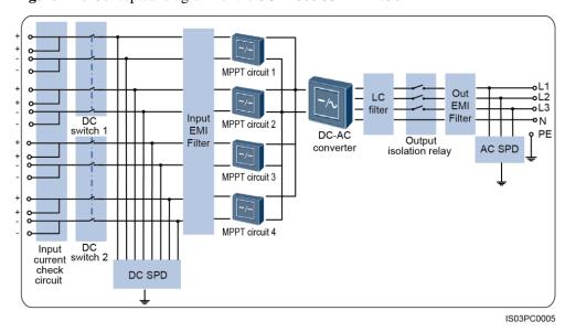
Figure 2-10 Conceptual diagram for the SUN2000-33KTL-A/36KTL
