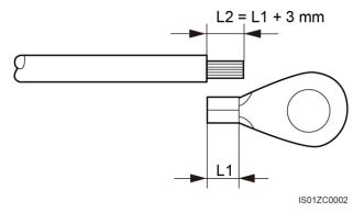
**Step 2** Insert the exposed core wires into the crimping area of the OT terminal and crimp them using hydraulic pliers, as shown in Figure 5-4.
