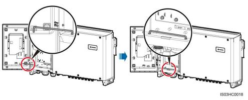
**Step 3** Close the maintenance compartment door. Tighten the two screws on the maintenance compartment door using a security torx wrench to a torque of 5 N m.
