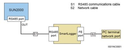
Figure 5-25 shows the communication mode for multiple SUN2000s.
