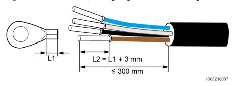
Figure 5-11 Five-core cable (including the ground cable and neutral wire)
