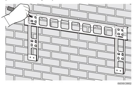
**Step 3** Drill holes using a hammer drill and install expansion bolts.
