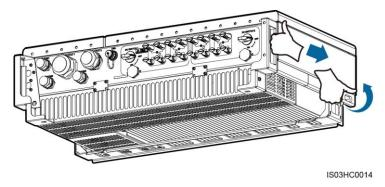
**Step 4** Run a rope that is strong enough to bear the SUN2000 through the lifting eyes and hoist the SUN2000.
