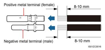
**Step 2** Insert the exposed area of the positive and negative power cables into the metal terminals of the positive and negative connectors respectively and crimp them using a crimping tool, as shown in Figure 5-18. Ensure that the cables are crimped tightly such that they cannot be pulled out by a force less than 400 N.
