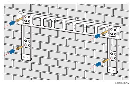
Figure 4-14 Securing a mounting bracket
