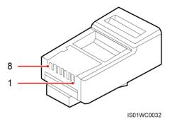
The FE communications cable is connected over standard network cables. A standard network cable can be 568A or 568B. The network cables used in the same PV grid-tied power
