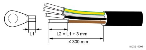
Figure 5-10 Four-core cable (excluding the ground cable but including the neutral wire)
