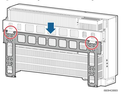
Figure 4-17 Mounting the SUN2000 onto the mounting bracket
