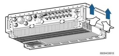
**Step 2** Lift the SUN2000 from the packing case and move it to the installation position with the help of multiple persons.
