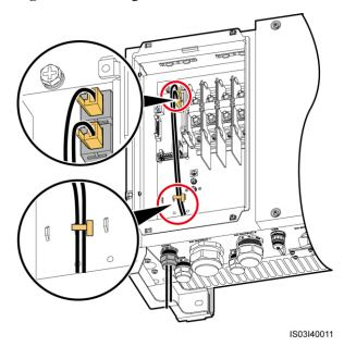
Figure 5-40 Binding communications cables
