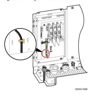
Figure 5-34 Binding communications cables
